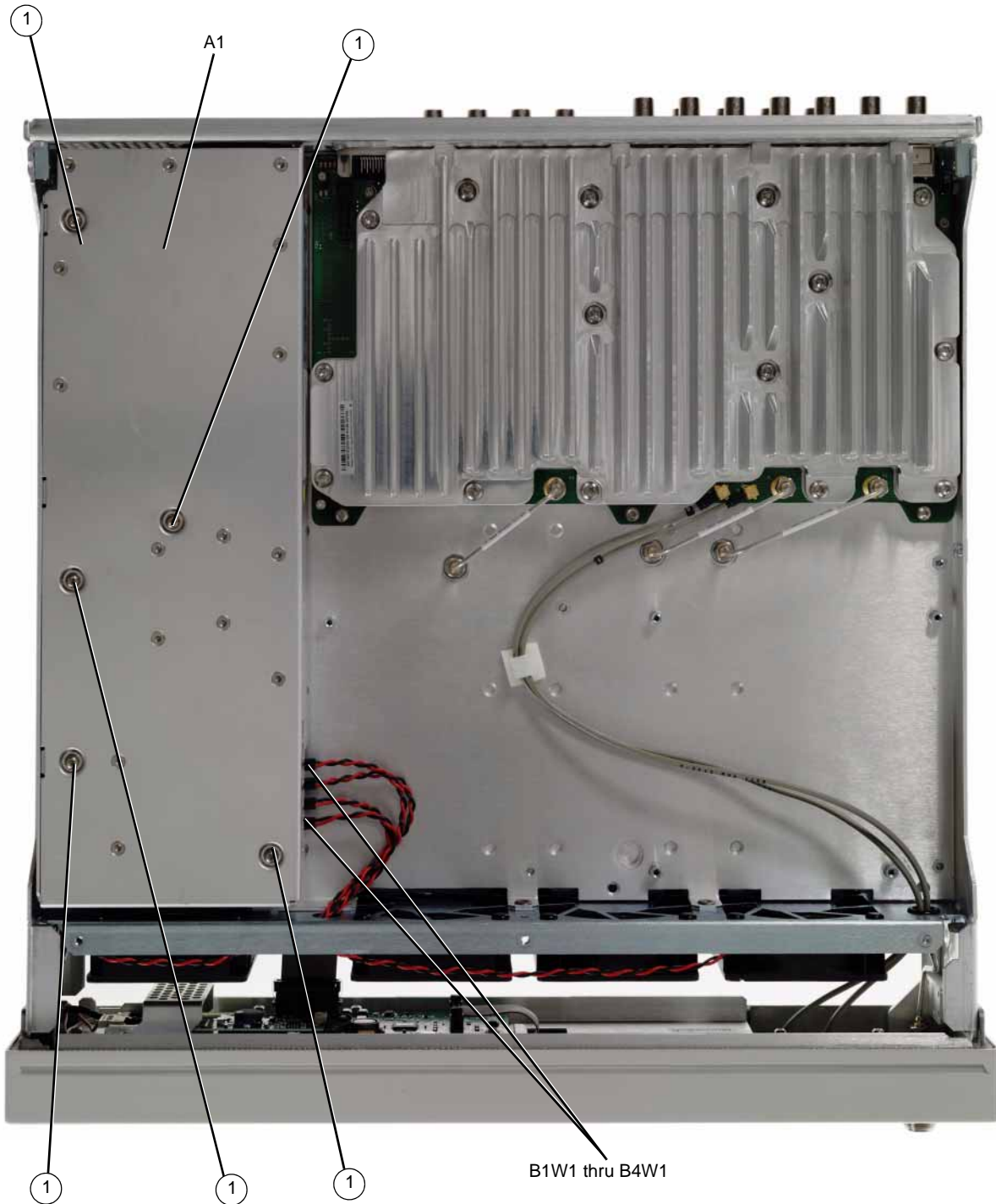
Figure 3-14 A1 Power Supply
